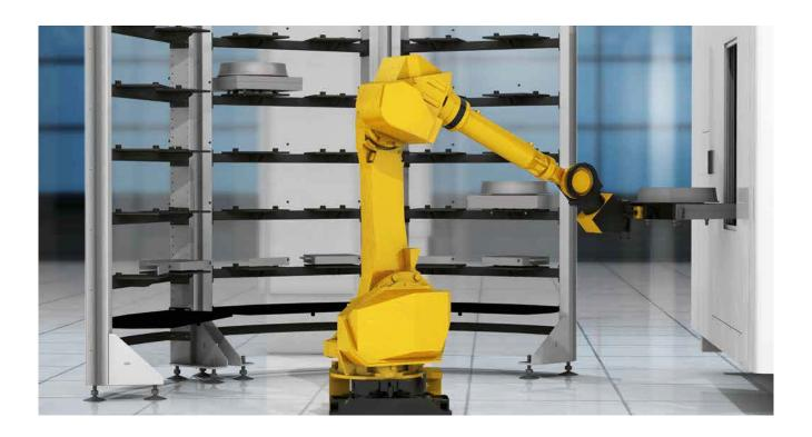
To underline our mutual commitment to providing innovative solutions to market leaders, GF Machining Solutions has filed a patent application for a new carrier concept. This flexible solution allows the user to position and locate build plates on the RPM and provides links to automated conventional machining processes. This concept contributes to a significant increase in automation possibilities and reduction of build plates costs.
