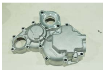
(The cooler cover to be inspected)
